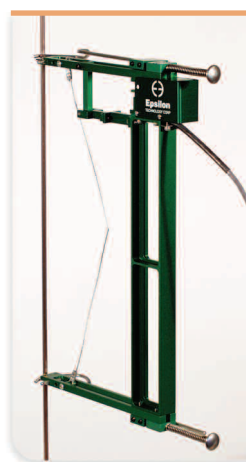
Model 3542L with 8 inch gauge length and ±0.4 inch measuring range
