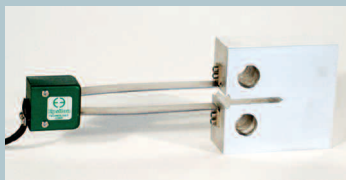
Model 3541-004M-120M with 4 mm gauge length and +12/-2 mm measuring range
