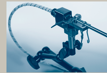
3640 High temperature 540 °C (1000 °F) capacitive based deflectometer. The model shown has 1 inch of measuring range.
