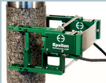
Model 3542RA1 extensometer with 50MM gauge length
