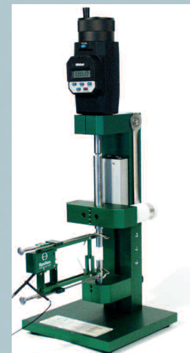
Model 3590 with Model 3542 axial extensometer
