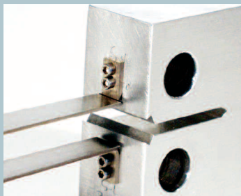
Model 3541-004M-120M attached to bolt-on knife edges
