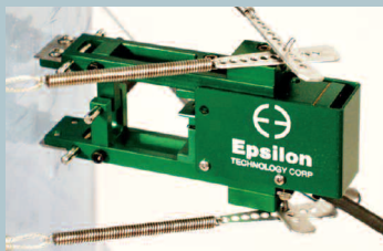
Model 3542 configured for a very large specimen diameter
