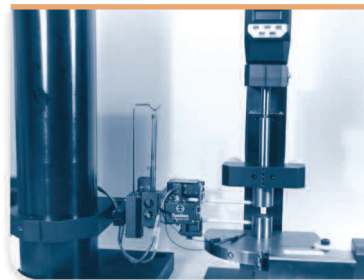
Model 3550HT extensometer with calibration stand
