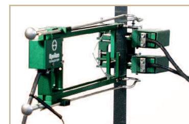
Models 3575AVG Transverse Used with Model 3542 extensometer.
