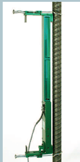
Model 3543 with 12 inch gauge length
