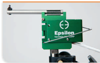
Model 3540 with 0.05 inch measuring range
