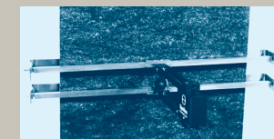
3542 on 250 mm Wide Special mounting for Model 3542 extensometer on 250 mm wide test samples.
