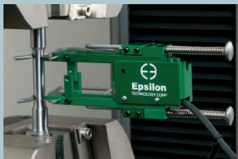
Model 3542 with 25 mm gauge length
