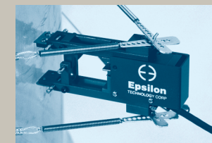
3542 on Very Large Sample Modification to Model 3542 extensometer for mounting on large diameter test samples.
