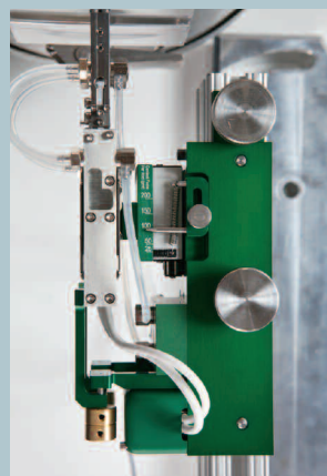
Model 3549 contact force scale for repeatable placement against test specimens
