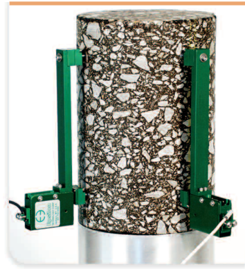
Model 3909-0400 with 4 inch gauge length
