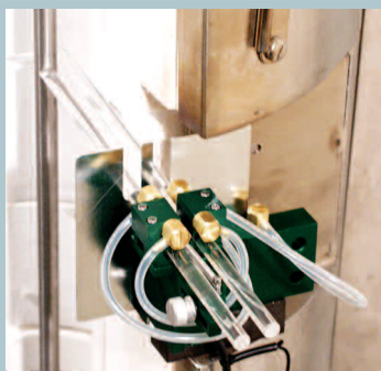
Model 3580 mounted to split furnace
