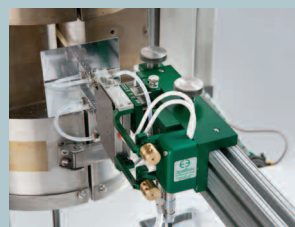
Model 3549 with 25 mm gauge length
