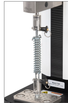
Tension spring testing
