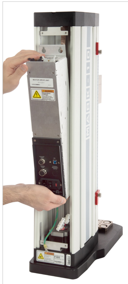
Removing the electronics module
